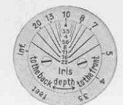
The helpful depth-of-focus scale
